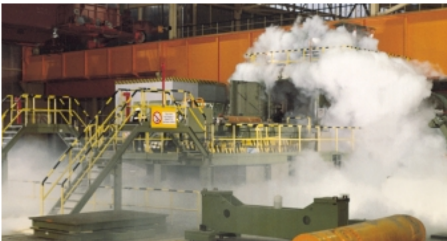
Discharge test of a rolling mill with CO 2
